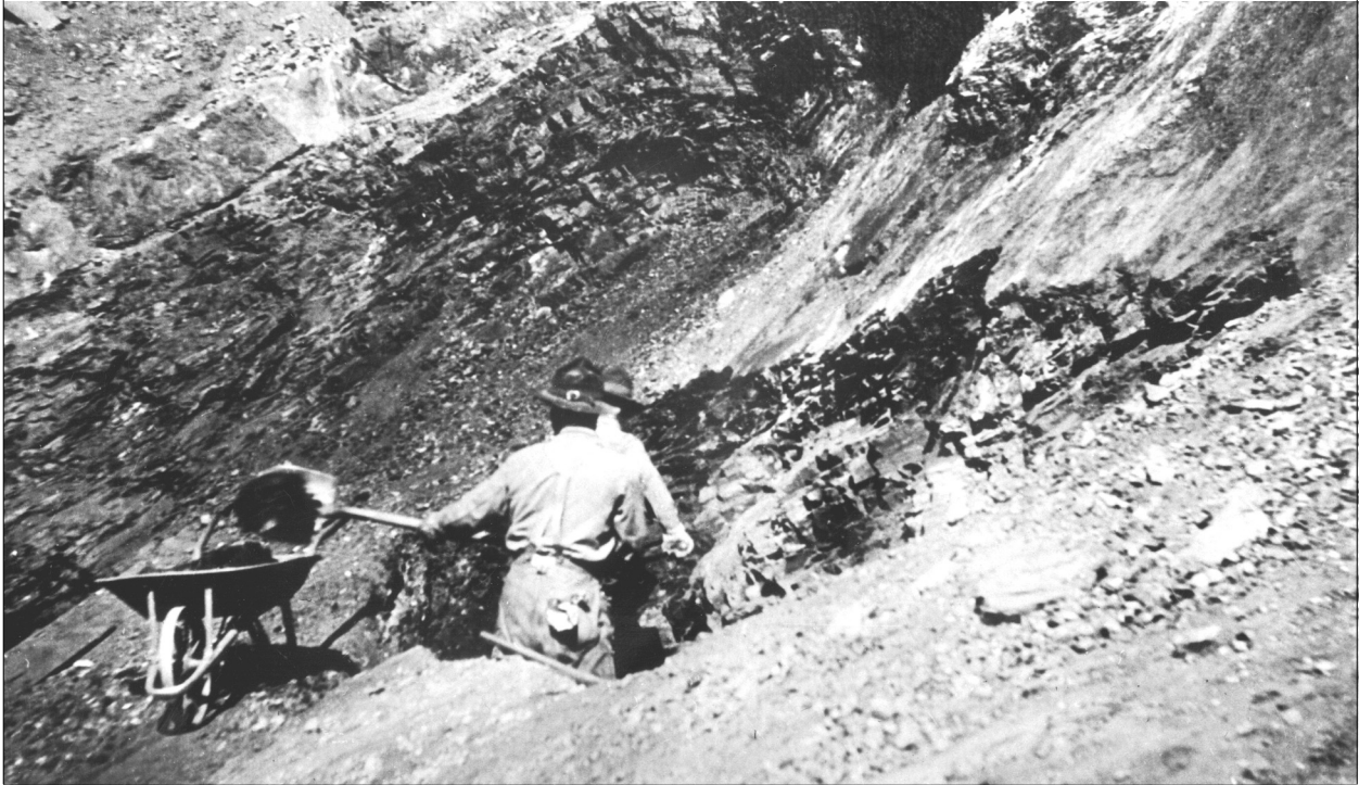
Figure 5. Black phosphate bed opened by surface stripping at Waterloo Mine. Photo by V. R. D. Kirkham, courtesy of the Idaho Geological Survey.
